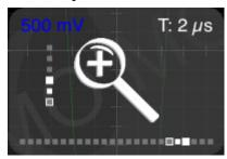
The blue number in the top left corner shows your volts per division and the white number in the top right corner shows the timescale. Focus on the right image. The two solid dots show where you're headed and the white outlined dot shows your current scale.
