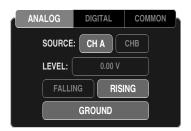
To navigate to an exact trigger level touch on next to the word LEVEL. The analog trigger level pick wheel should then appear.
